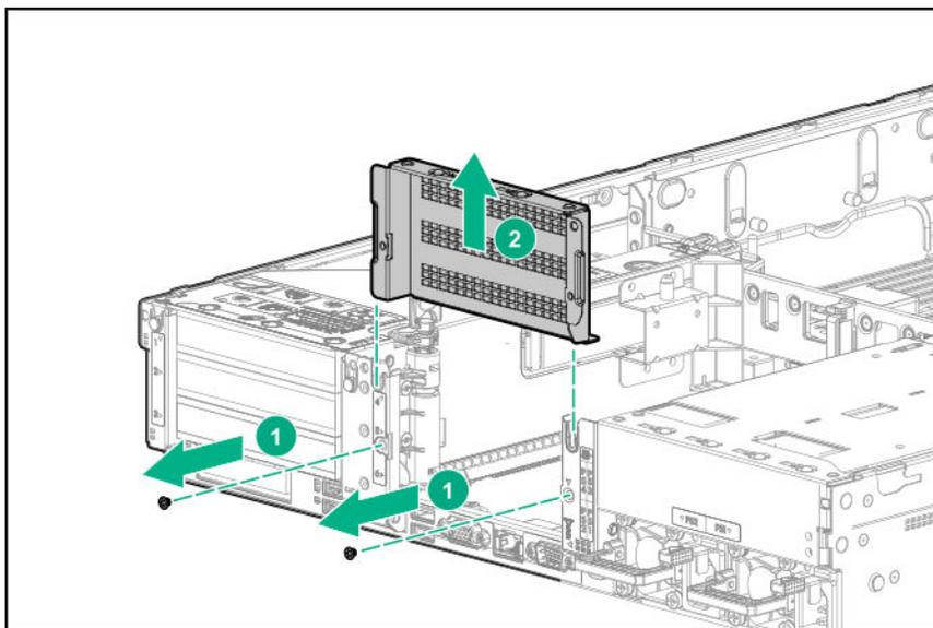
6. Remove the power cage blank.
