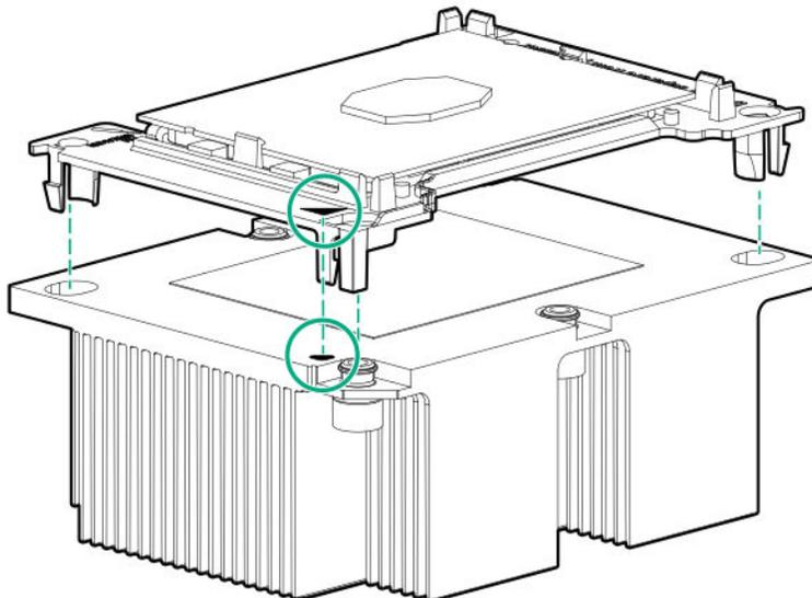
13. Install the processor heatsink assembly:
