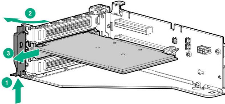
8. If installed, remove the riser board installed in the riser cage.
