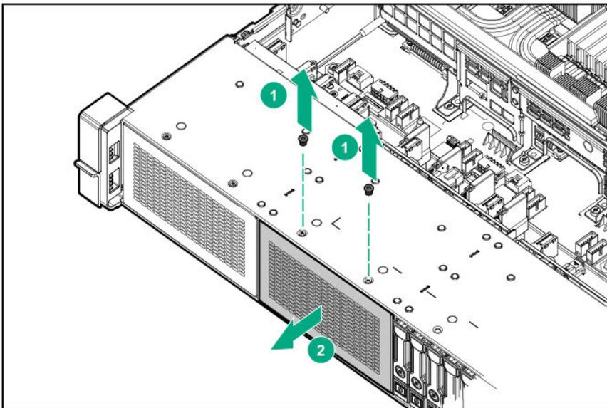
8. If drive blanks are installed in the drive cage assembly, remove the drive blanks. Retain the drive blanks for use in empty drive bays.
