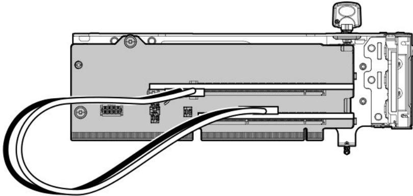
14. Install the riser cages into the server, and observe the following cable routing:
