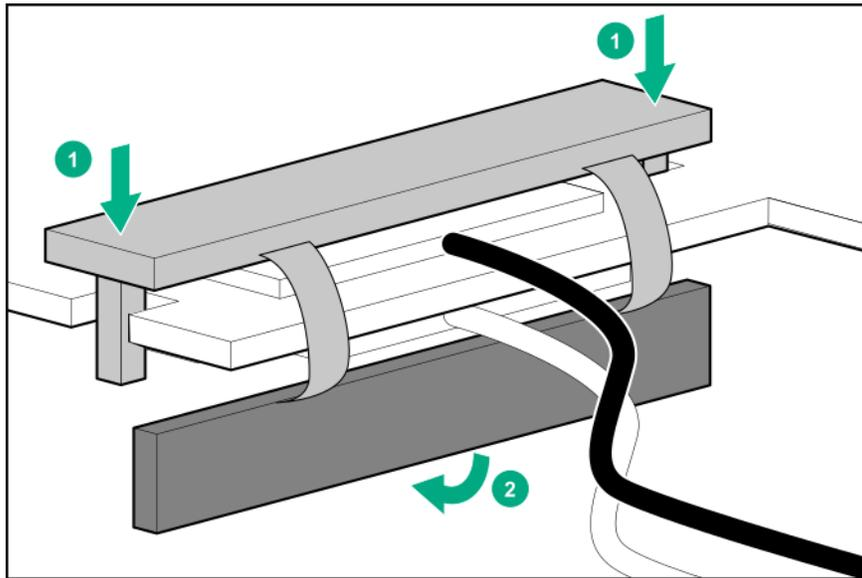
10. Thread the auxiliary cables through the second retention clip.
