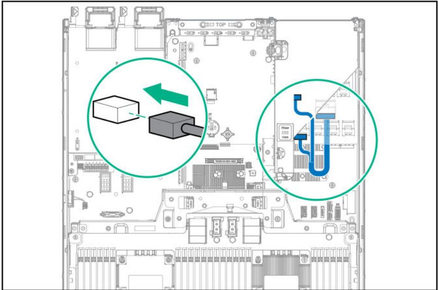
**13.** Connect the cables to the drive cage backplanes:
