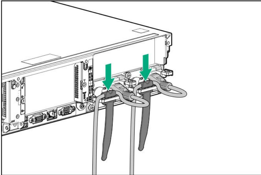
5. Secure the cables to the cable management arm.
