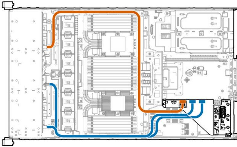
Quad slimline riser installed in the secondary PCIe riser cage
