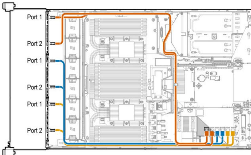
From the drive cage backplane to the controller in the secondary PCIe riser cage
