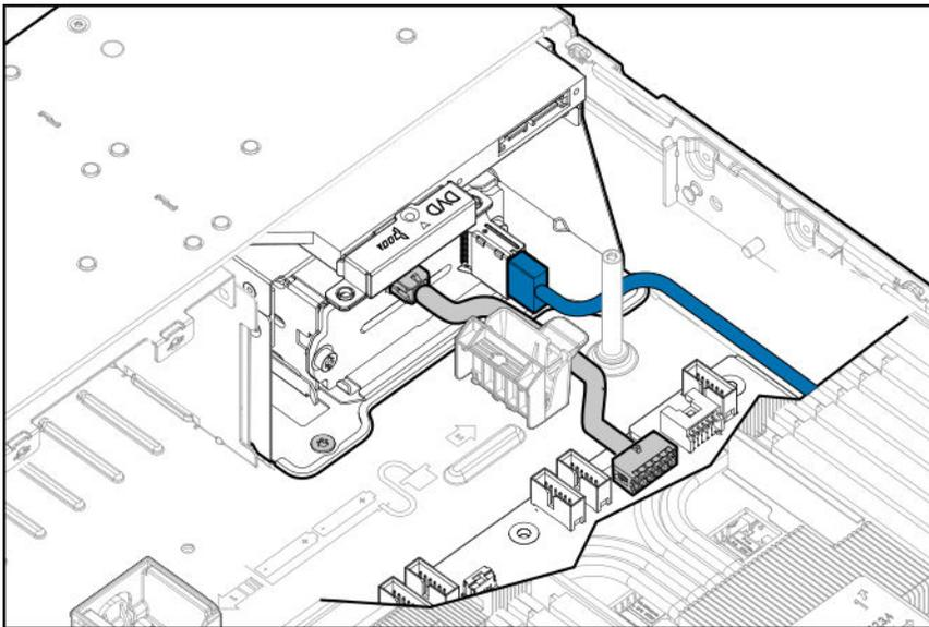
15. Route and connect the cables depending on the types of drives installed and the server configuration. For more information, see **Cabling** on page 162.
