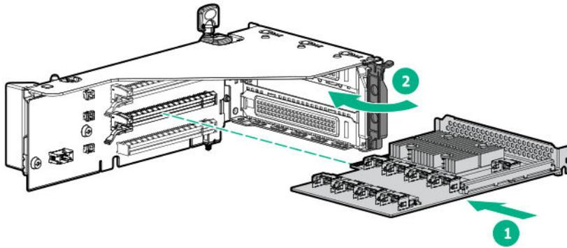
11. Install the primary PCIe riser cage ([Installing the primary PCIe riser cage](#) on page 60).
