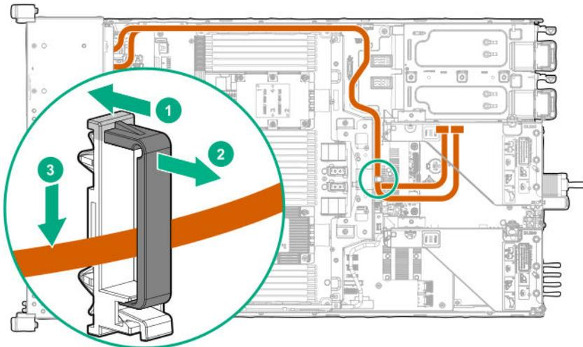
Connected to the tertiary PCIe riser board
