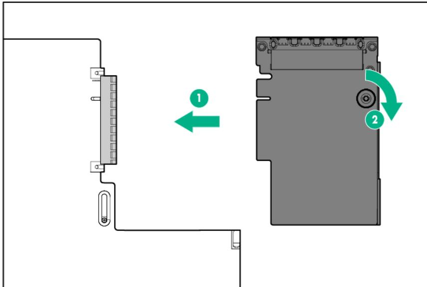
8. Install the primary PCIe riser cage (**Installing the primary PCIe riser cage** on page 60).
