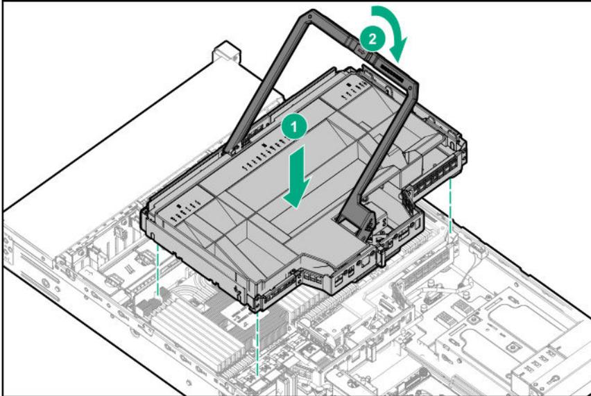
7. Install the access panel (**Installing the access panel** on page 56).
