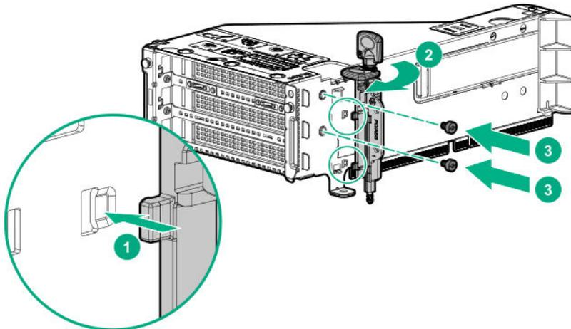
8. Install an expansion board into the secondary PCIe riser cage (**Installing an expansion board** on page 99).
