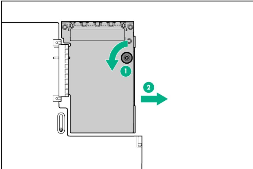
7. Install the FlexibleLOM adapter.
