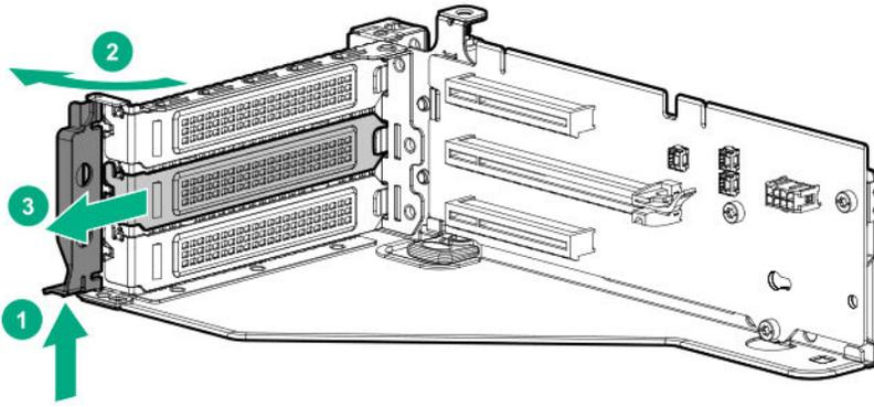
7. Install the GPU card into the riser.
