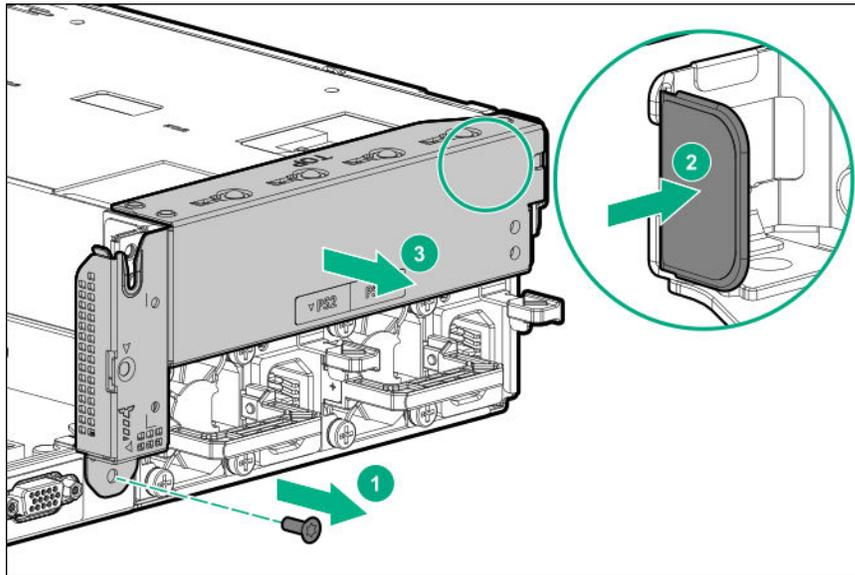
7. Install the power supply cage.
