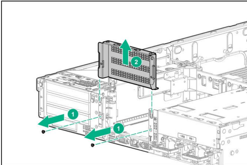
6. When installing the secondary PCIe riser cage for the first time, remove the fastener from the riser cage.
