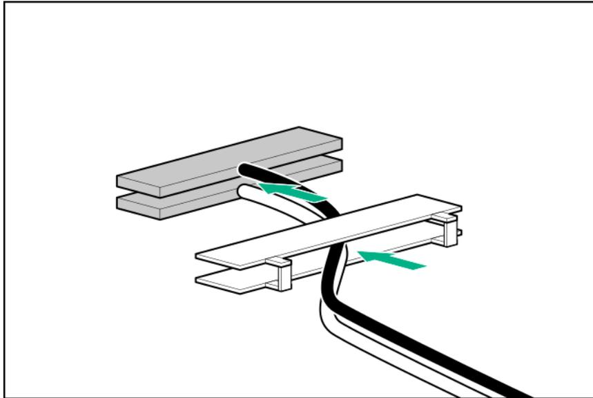
8. Open the cable latch door, connect the auxiliary card cables to the adapter ports so that the golden side of the cable connector is on the top, and then close the cable latch door.
