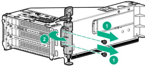
7. Install the additional fastener supplied with the option kit onto the riser cage.
