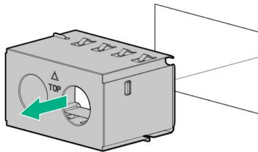
3. Install the power supplies into power supply bays 1 and 2 until each click into place.
