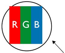
One dot = One Pixel; consists of three sub-pixels of Red, Green, and Blue.
