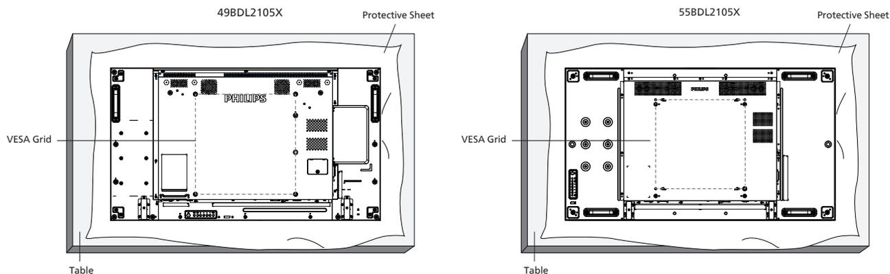
1. Spread a protective sheet which was wrapped around the display when it was packed on a flat surface. Lay the display face-down on the protective sheet to facilitate your operation without scratching the screen.
