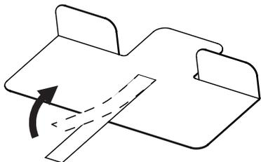
2. Stick the gap pad to the top surface of the display where another display will be stacked. Apply 2 gap pads on the top surface.
