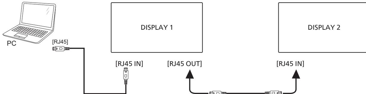
Connect laptop [USB] to adaptor and connect to [Control IN] of DISPLAY 1, connect the [Control OUT] connector of DISPLAY 1 to the [Control IN] connector of DISPLAY 2.
