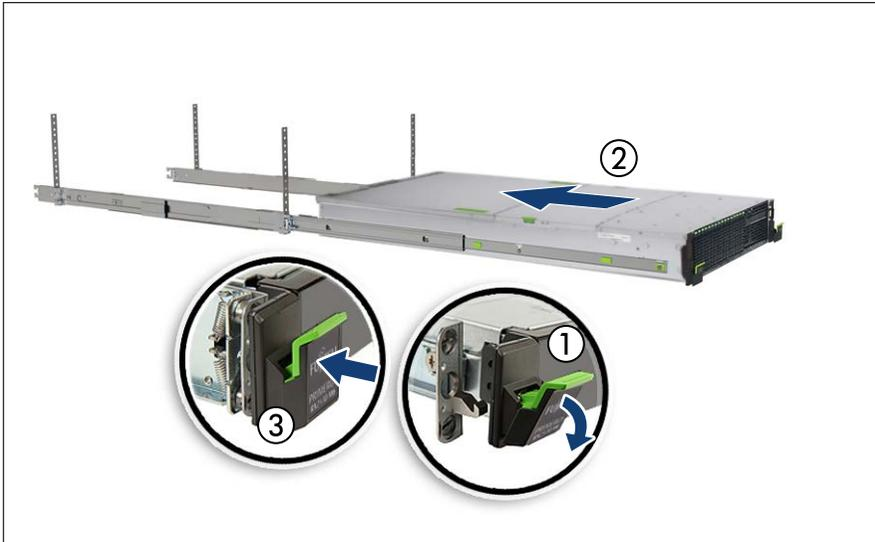
Figure 24: Sliding the server into the rack
