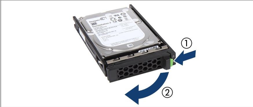
Figure 37: Opening the locking lever
