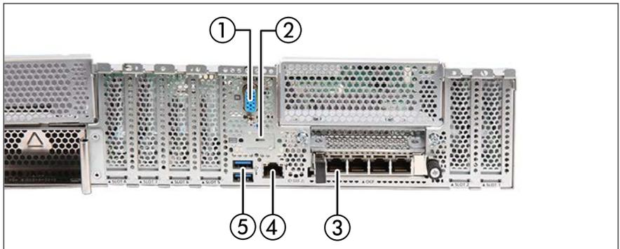
Figure 16: Connectors on the server rear
