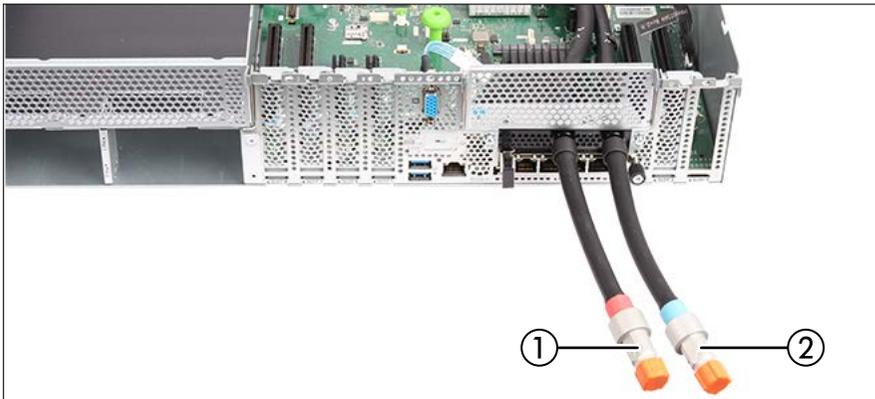
Figure 17: Quick connectors for liquid cooling
