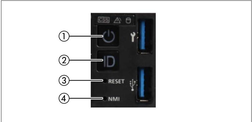
Figure 11: Controls on the COP
