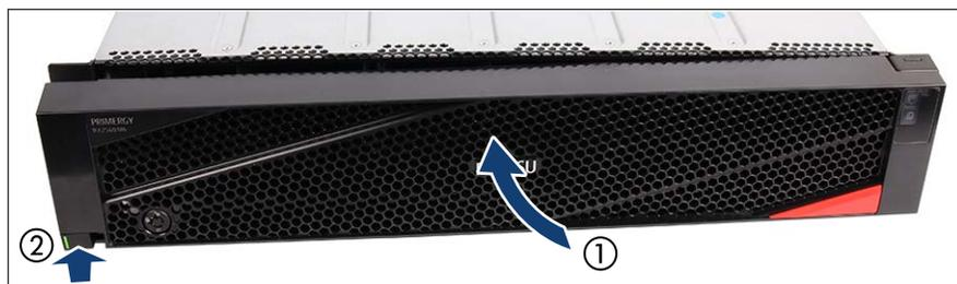
Figure 29: Installing the front cover with lock
