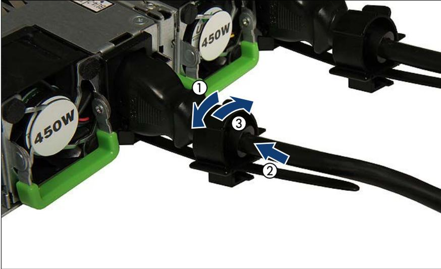
Figure 26: Locking the cable clamp of a PSU
