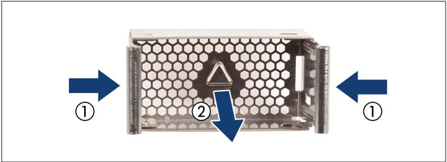
Figure 42: Removing the dummy cover
