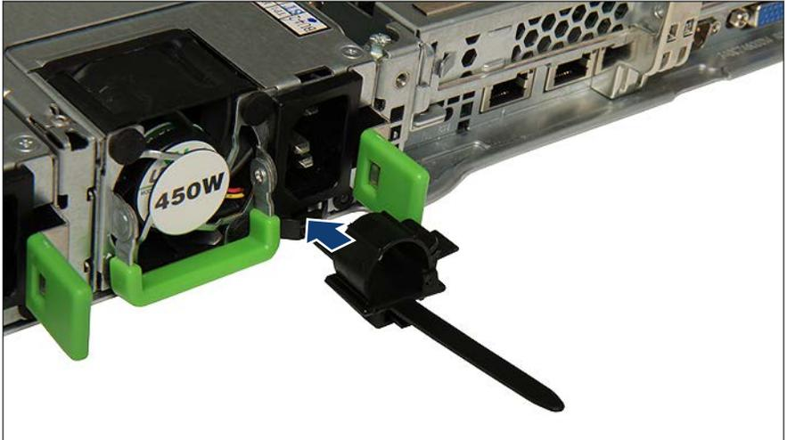
Figure 45: Installing the cable clamp
