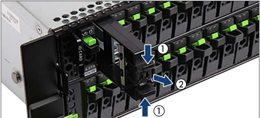
Figure 39: Removing an EDSFF dummy module
