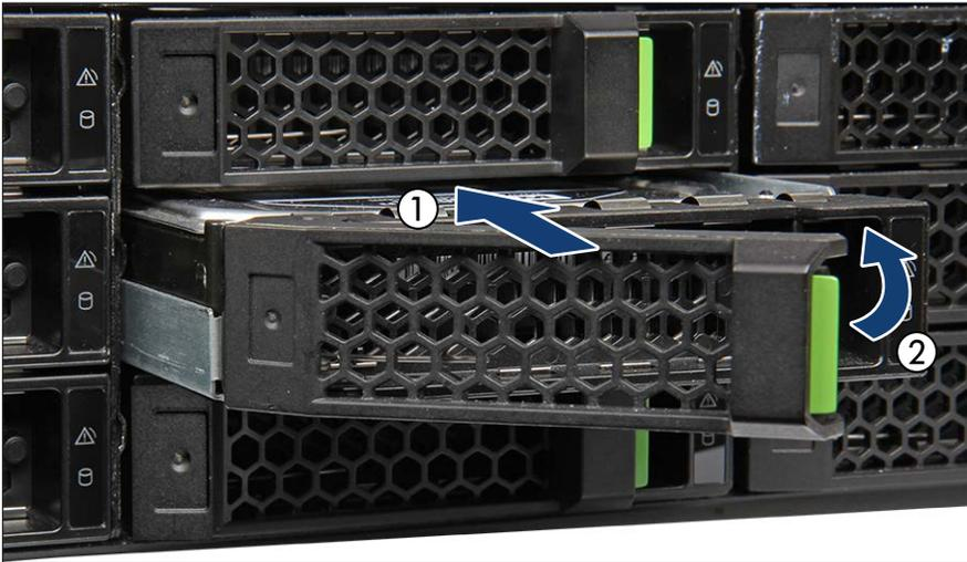
Figure 35: Installing the 3.5-inch HDD module
