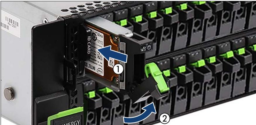
Figure 41: Installing the EDSFF SSD module
