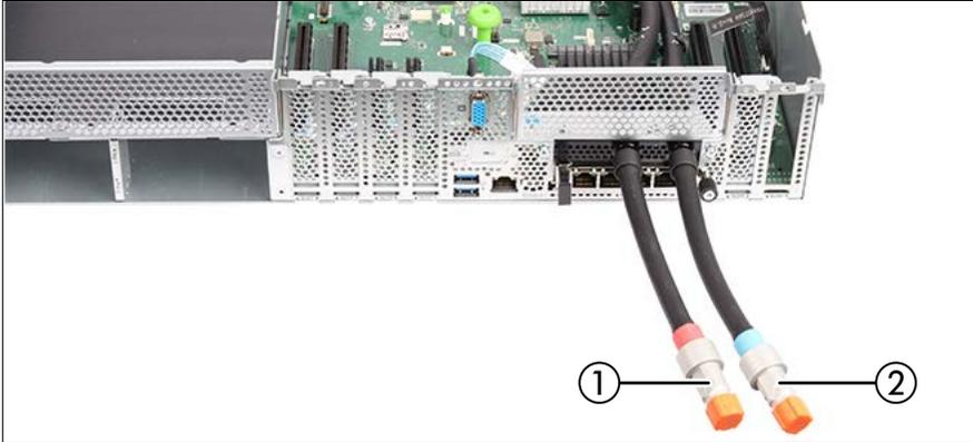
Figure 25: Quick connectors for LC
