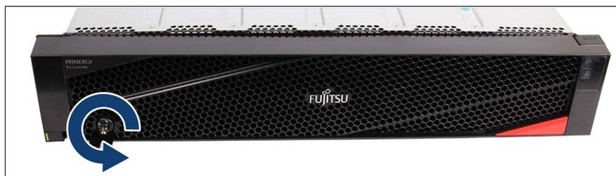
Figure 30: Turning the key
