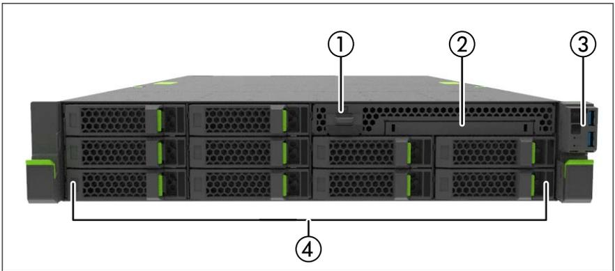
Figure 1: Front side 10x 3.5-inch HDDs
