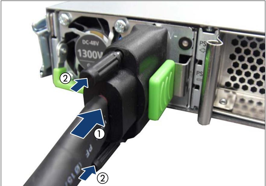
Figure 27: Connecting the server to the DC voltage - example DC PSU -48 V
