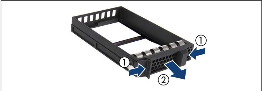
Figure 33: Removing the 3.5-inch dummy module
