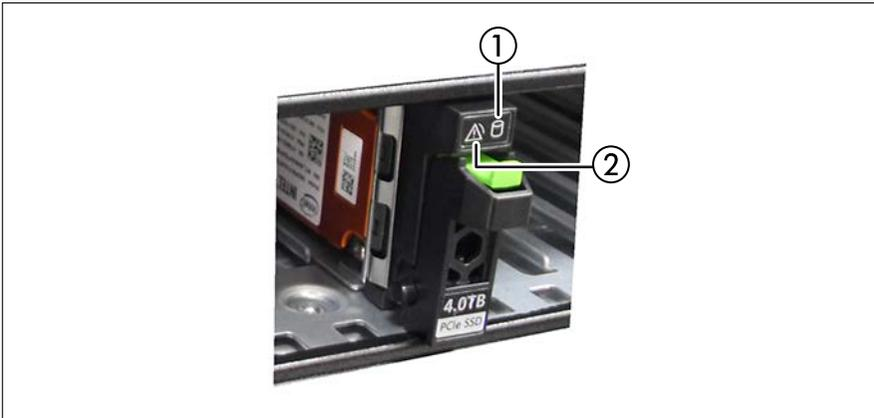
Figure 15: Indicators on an EDSFF SSD module
