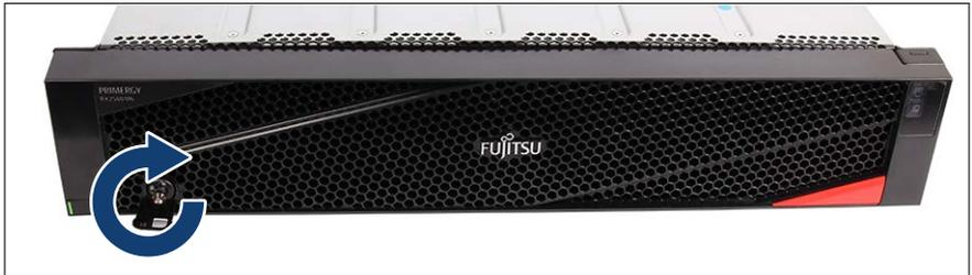
Figure 31: Turning the key
