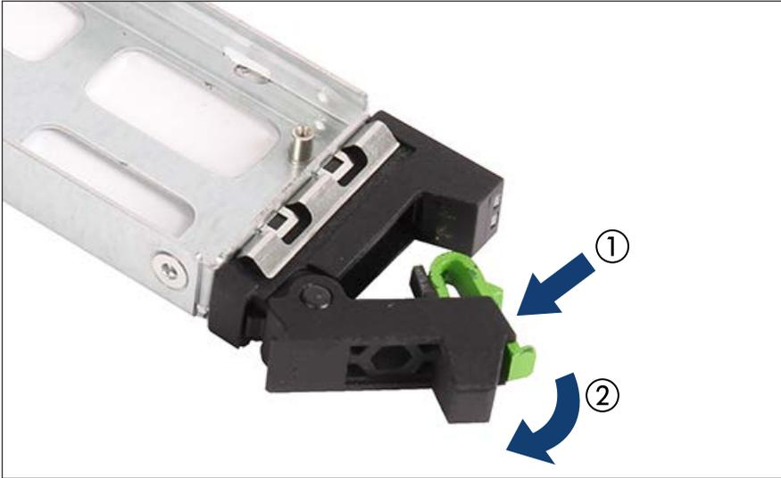
Figure 40: Opening the locking lever
