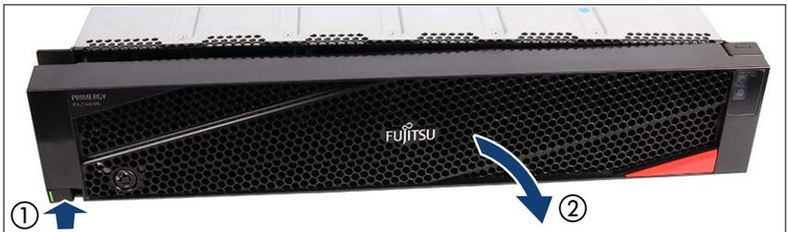
Figure 32: Removing the front cover
