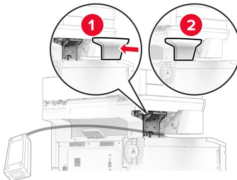
**Note:** Secure the power supply properly.
