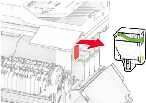
**6** Remove the imaging kit.
