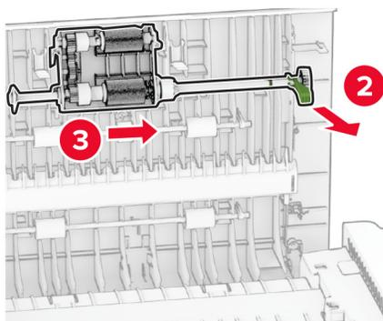
**3** Remove the ADF separator roller.
