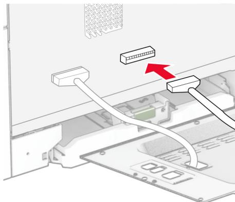
**10** Attach the controller board shield, and then install the screws.
