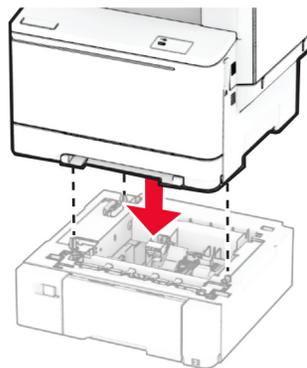
**Note:** To avoid invalid configuration, when installing both the 550-sheet tray and 650-sheet tray, always place the 550-sheet tray below the 650-sheet tray.
