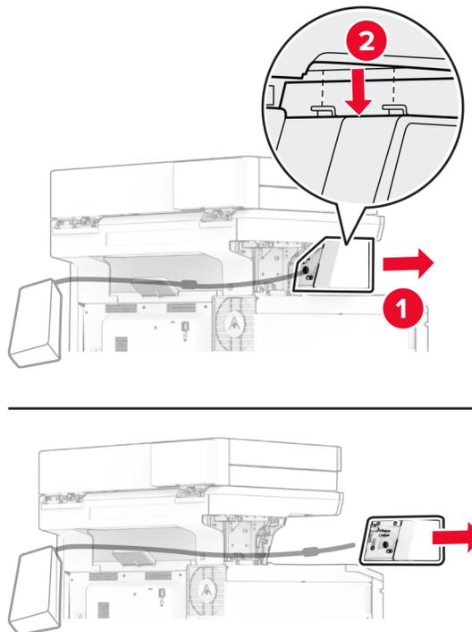
**6** Remove the used power supply.
