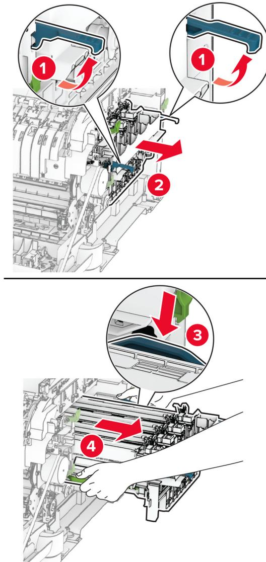
**7** Remove the used developer unit.
