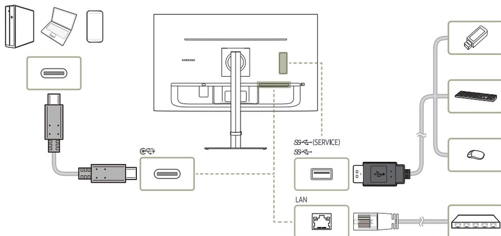
Using the product as a hub, connect and use various source devices with the product at a time.
