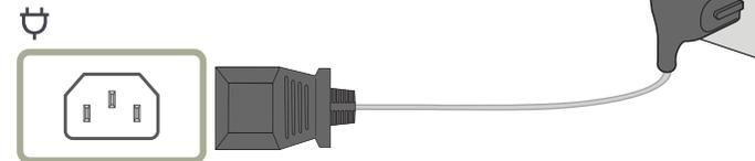
To use the product, connect the power cable to a power outlet and the power port on the product.
