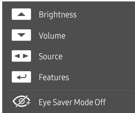
— The Direct Key Guide screen shows if **Eye Saver Mode** is enabled. (**Off, Low, High**)
