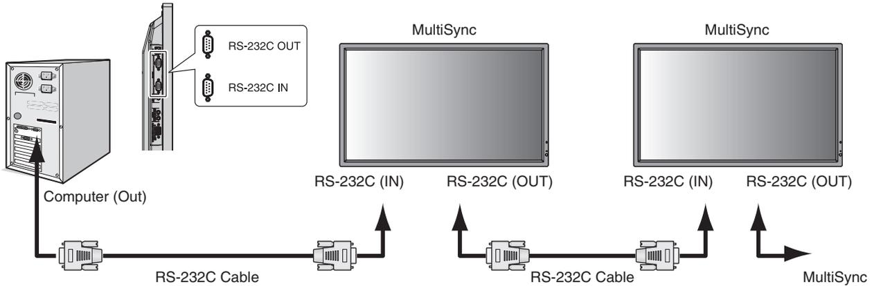
**NOTE:** If your computer is equipped only with a 25-pin serial port connector, a 25-pin serial port adapter is required. Contact your dealer for details. Check the “ID=ALL REPLY” setting in “EXTERNAL CONTROL”.
