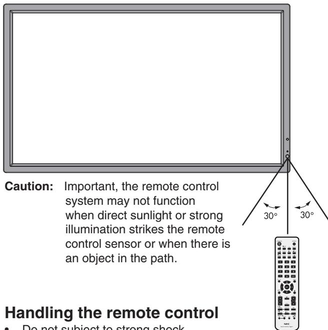
**Caution:** Important, the remote control system may not function when direct sunlight or strong illumination strikes the remote control sensor or when there is an object in the path.
