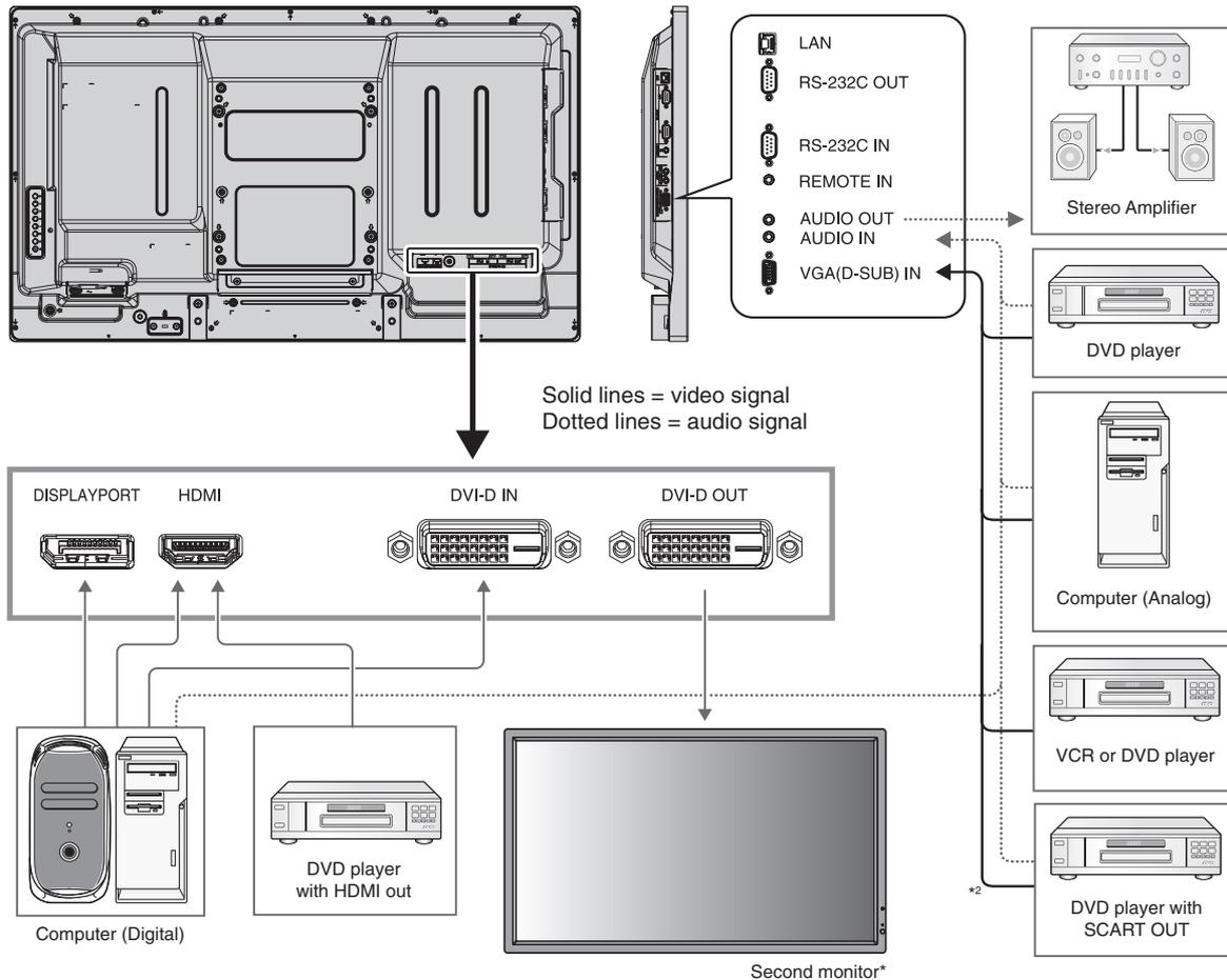
\*: Multiple monitors that are daisy-chained have a limit to the connectable monitors.
