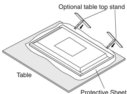
**NOTE:** Install the stand in the direction of the arrow which is imprinted on the surface of the stand. Use the ST-322 for V323-3.
