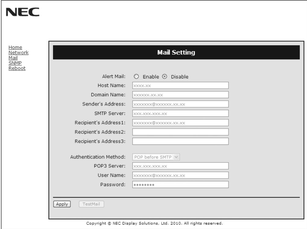
This option notifies your computer of an error message via e-mail when using wired LAN. An error message notification will be sent when an error occurs in the monitor.
