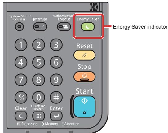
If print data is received during Sleep, the machine automatically wakes up and starts printing. Also when fax data arrives while the machine is in Sleep, the machine automatically wakes up and starts printing.
