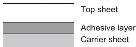
Labels consist of three layers as shown in the illustration. The adhesive layer contains materials that are easily affected by the force applied in the machine. The carrier sheet bears the top sheet until the label is used. This composition of labels may cause more problems.
