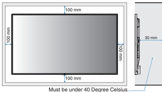
Allow adequate ventilation or provide air conditioning around the monitor, so that heat can properly dissipate away from the unit and the mounting equipment; especially when you use monitors in a multiple screen configuration.
