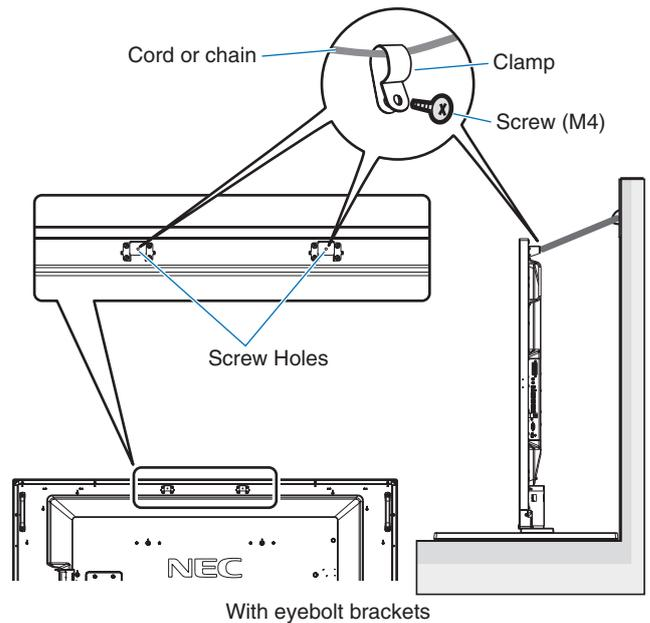
Before attaching the LCD monitor to the wall, make sure that the wall can support the weight of the monitor.
