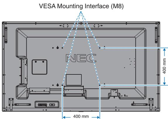
Mounting accessories can be attached with the monitor in the face down position. To avoid damaging the front face, place the protective sheet on the table underneath the LCD monitor. The protective sheet was wrapped around the LCD monitor in the original packaging. Make sure there is nothing on the table that can damage the monitor.
