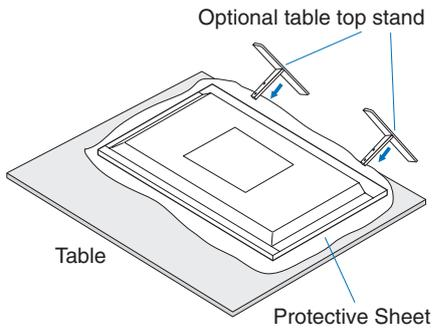
**NOTE:** Install the stand in the direction of the arrow which is imprinted on the surface of the stand. Use the ST-801.
