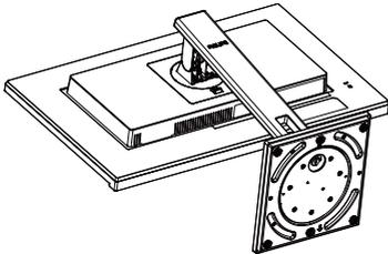
3. While keeping the release button pressed, tilt the base and slide it out.
