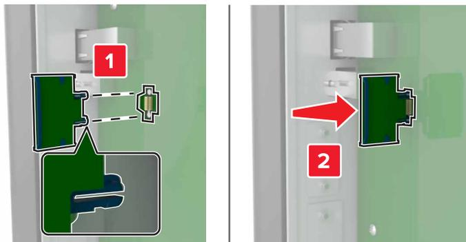
**Note:** The entire length of the connector on the card must touch and be flush against the controller board.
