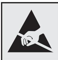
This symbol identifies static-sensitive parts. Do not touch the areas near these symbols without first touching a metal surface in an area away from the symbol.
