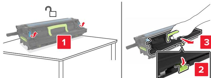
**6** Unpack the new developer unit, and then remove the packing material.
