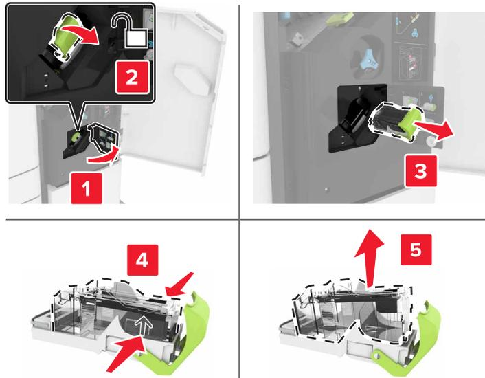
**3** Unpack the new staple cartridge, and then remove the tape.
