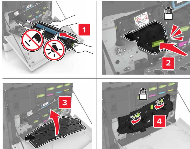
**9** Insert the waste toner bottle.
