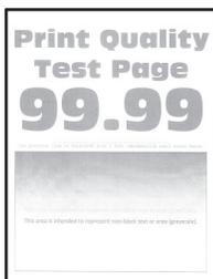
**Note:** Before solving the problem, print the Print Quality Test Pages. From the control panel, navigate to **Settings > Troubleshooting > Print Quality Test Pages**. For non-touch-screen printer models, press
