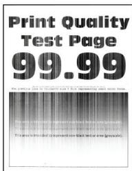
**Note:** Before solving the problem, print the Print Quality Test Pages. From the control panel, navigate to **Settings > Troubleshooting > Print Quality Test Pages**. For non-touch-screen printer models, press
