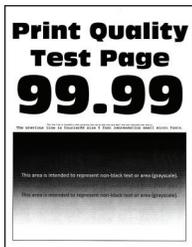
**Note:** Before solving the problem, print the Print Quality Test Pages. From the control panel, navigate to **Settings > Troubleshooting > Print Quality Test Pages**. For non-touch-screen printer models, press
