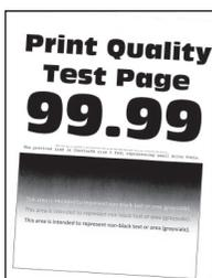
**Note:** Before solving the problem, print the Print Quality Test Pages. From the control panel, navigate to **Settings > Troubleshooting > Print Quality Test Pages**. For non-touch-screen printer models, press
