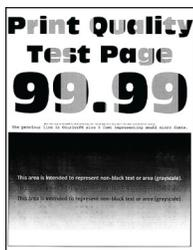
**Note:** Before solving the problem, print the Print Quality Test Pages. From the control panel, navigate to **Settings > Troubleshooting > Print Quality Test Pages**. For non-touch-screen printer models, press
