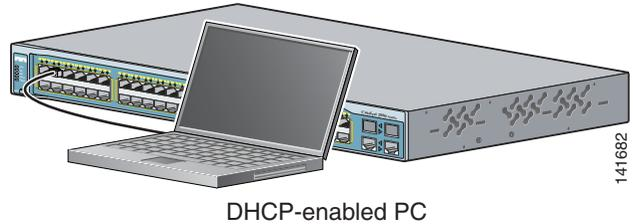
**Step 8** Verify that the LEDs on both Ethernet ports are green.
