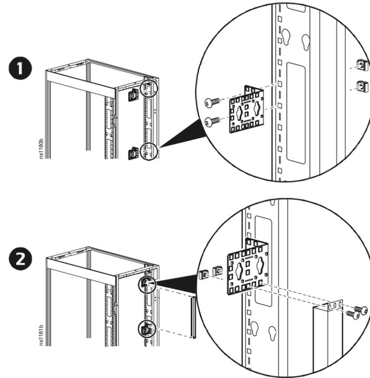
**Additional installation option attaching brackets together**
