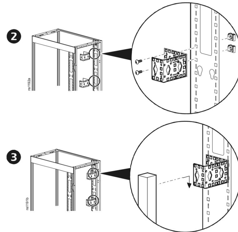
**Vertical rack-mount equipment installation—vertical mounting flanges**
