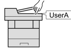
Access are in three levels - "User", "Administrator", and "Machine Administrator". The security levels can be modified only by the "Machine Administrator".
