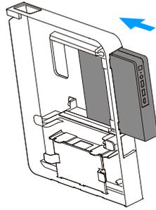
**Figure 15. Insert the OptiPlex personal computer**
