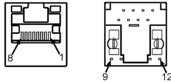
**Figure 10.** RJ45 connector
