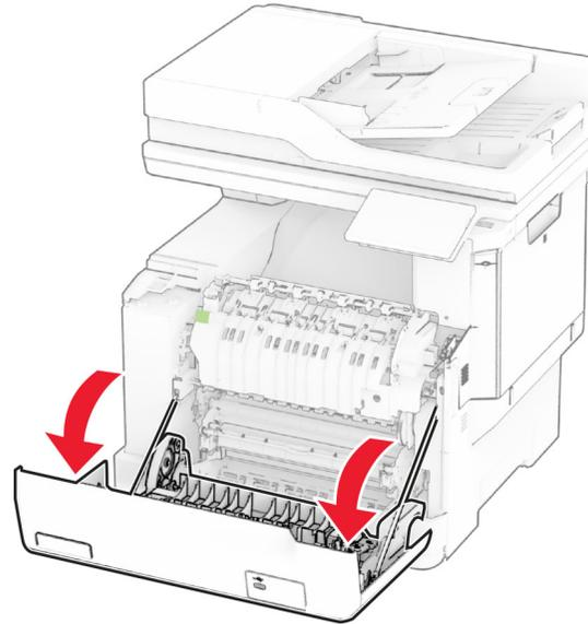
2 Open the fuser access door, and then remove the jammed paper.
