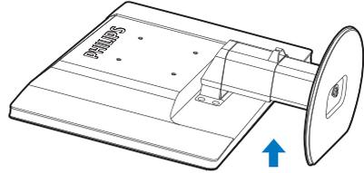
3. Release the lock of base stand then pull the base stand away from the base column.
