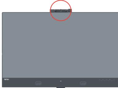
Slide the camera shutter open or close to enable/disable the camera.
