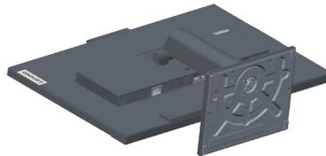
Step 3: Remove the base and stand from the monitor, refer to “Detaching the monitor base and stand” on page 2-11.
