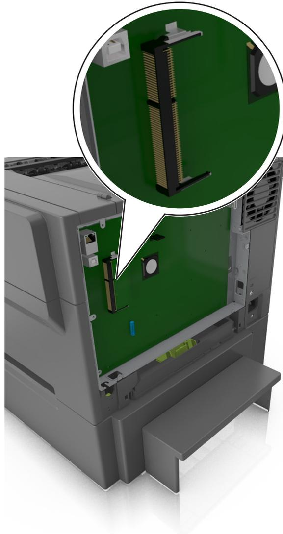
**Warning—Potential Damage:** Controller board electronic components are easily damaged by static electricity. Touch something metal on the printer before touching any controller board electronic components or connectors.
