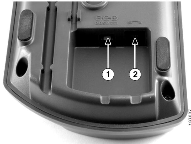
**Figure 1** Cisco SPA 301 Phone Power and Handset Connections
