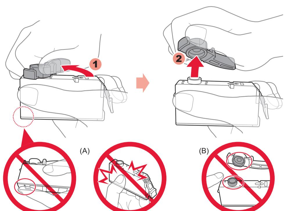
2 Twist and remove the orange cap.
