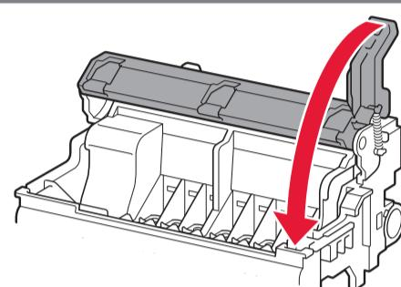
6 Lower the Print Head Lock Lever completely.
