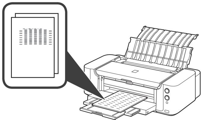
When the second page of the pattern is printed, Print Head Alignment is complete.
