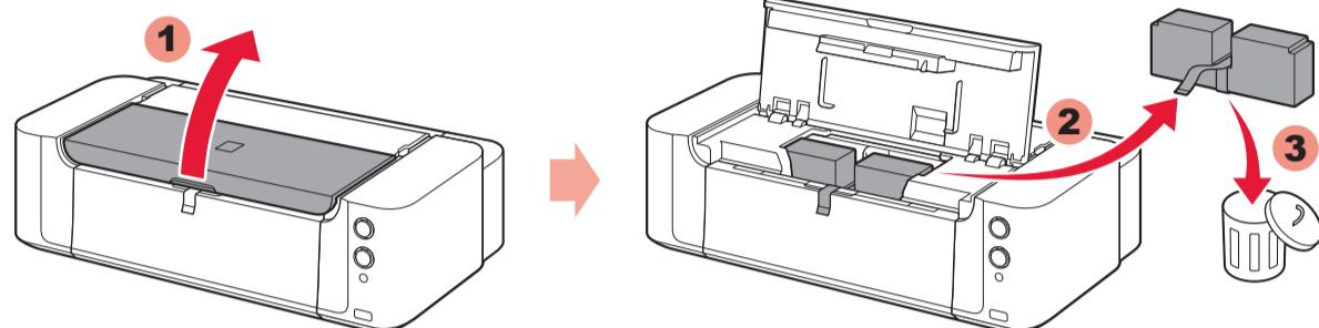
1 Open the Top Cover, then remove the orange tape and protective material.
