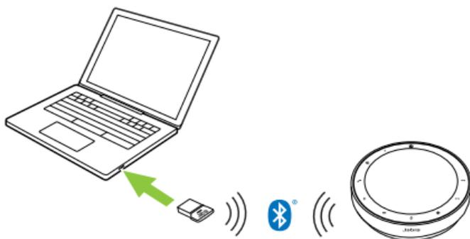
For the speakerphone to work correctly, you may need to set the Jabra Link 380 Bluetooth adapter as the playback and recording device in your operating system audio settings and in the video conferencing tool (Microsoft Teams, Zoom, Cisco Webex, etc.) audio settings.
