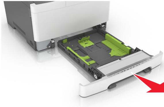
**2** If the paper is longer than letter-size paper, then push the length guide tab at the back of the tray to extend it.
