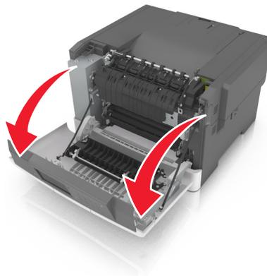
3 Slide the release latch on the right side of the printer, and then open the top door.
