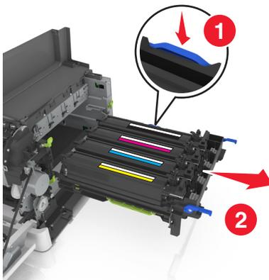
**8** Remove the used developer unit.
