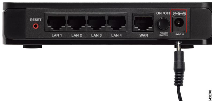
**STEP 7** On the Cisco RV180/RV180W, push in the ON/OFF power button.
