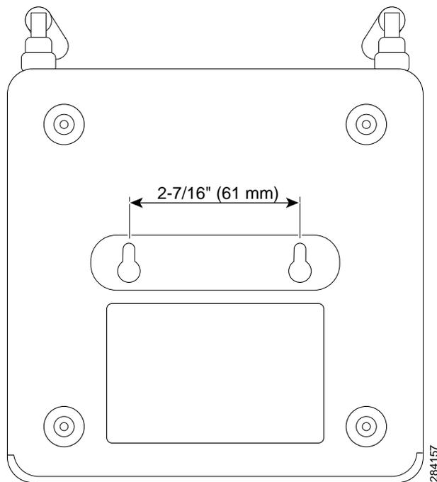
**STEP 4** Place the firewall wall-mount slots over the screws and slide the firewall down until the screws fit snugly into the wall-mount slots.
