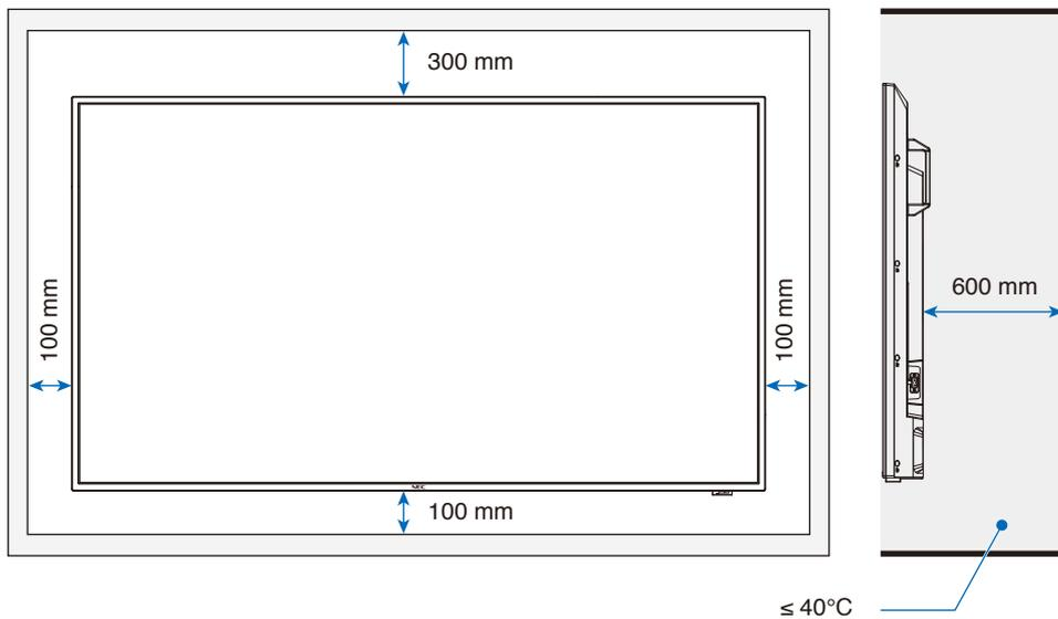
**NOTE:** The maximum environmental operating temperature of the monitor is 40 °C. This monitor has internal temperature sensors.
