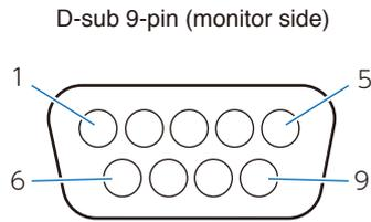
This monitor uses RXD, TXD and GND lines for RS-232C control.
