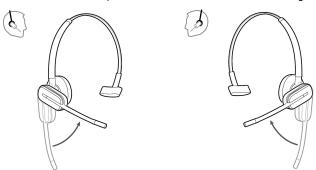
3 To optimize the position of the headset, push the headset in so the microphone is close to your mouth.
