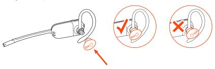
**NOTE** Ensure the large end of the eartip points to the microphone.
