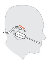
With a finger on the headset indicator light, push in until the microphone rests as close to your cheek as possible without touching.
