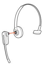
2 Rotate the headset up. The headband can be worn on the right or left side.
