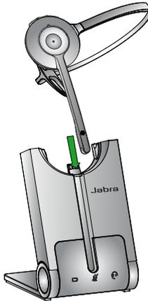
Dock the headset. When docked correctly the headset battery will begin charging, if needed. Charge for 20 minutes or until the battery indicator on the base
