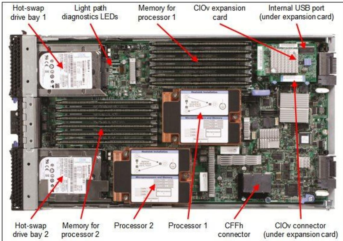
Figure 3. Top view of the IBM BladeCenter HS23E
