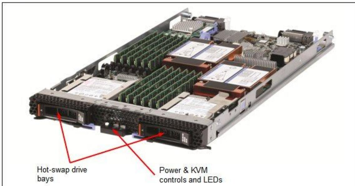
Figure 2. Front view of the IBM BladeCenter HS23E
