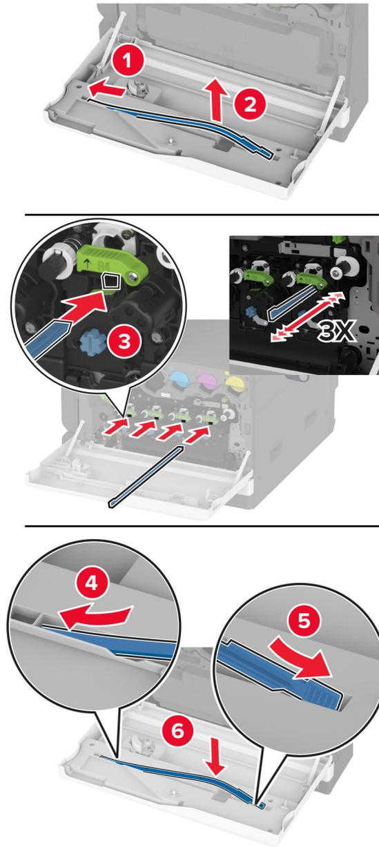
**7** Put the printhead wiper back into place.
