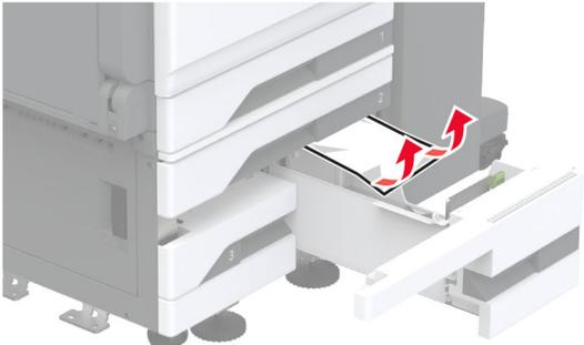
**6** In tandem trays, pull out handle C, and then open the inner cover.
