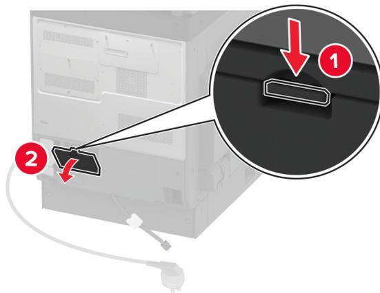
**9** Connect the tray connector to the printer, and then attach the cover.
