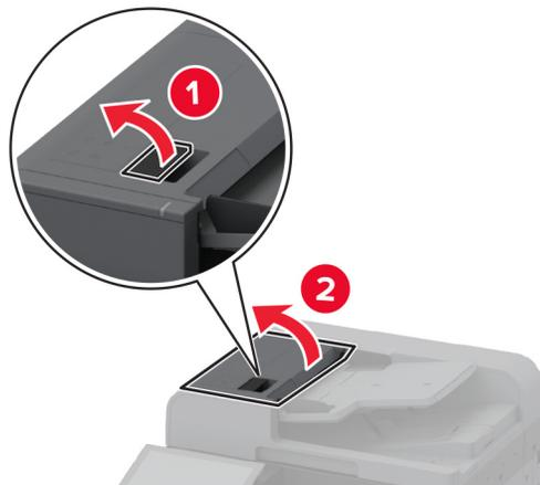
**3** Remove the separator roller cover.
