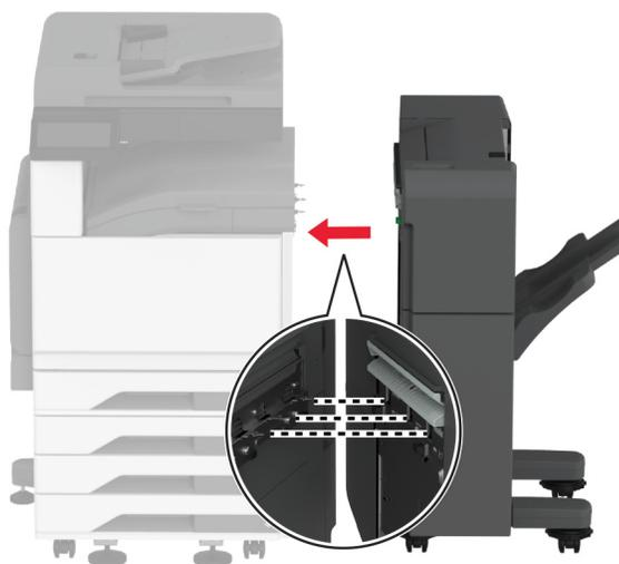
**14** Adjust the leveling screws to make sure that all sides of the finisher have the same height with the printer.
