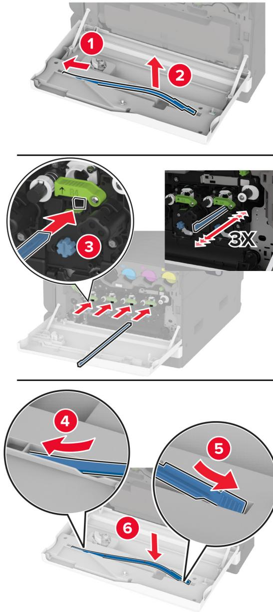
**7** Put the printhead wiper back into place, and then close the front door.
