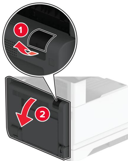
9 Open door C, and then remove the jammed paper.
