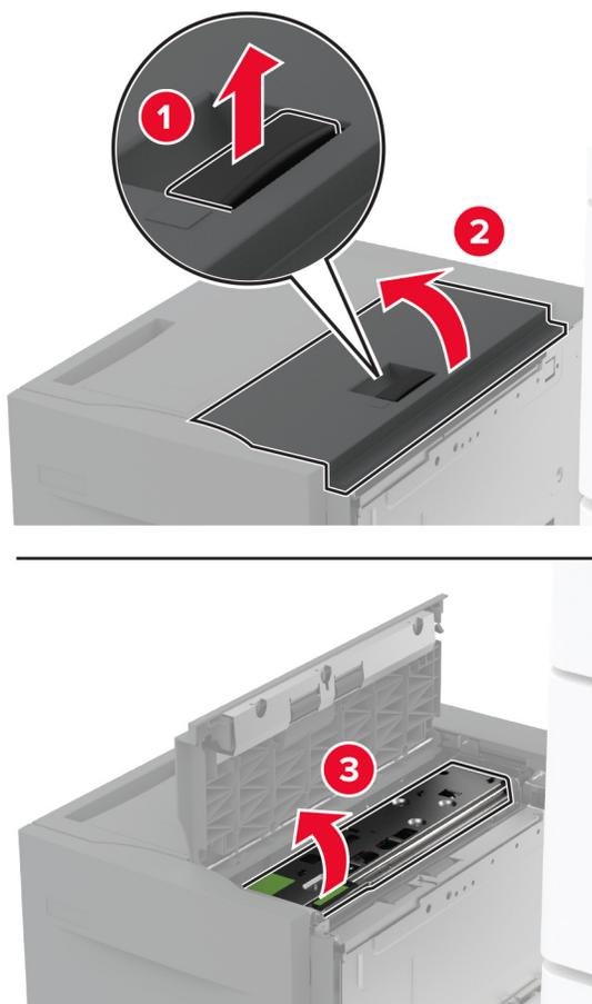
4 Locate and remove the used roller kit.
