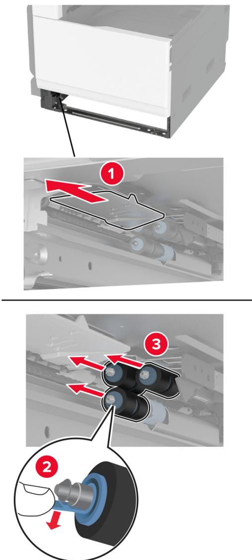
**4** Apply water to a soft, lint-free cloth, and then wipe the feed rollers.
