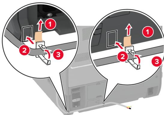
**13** Connect the finisher cable to the printer.
