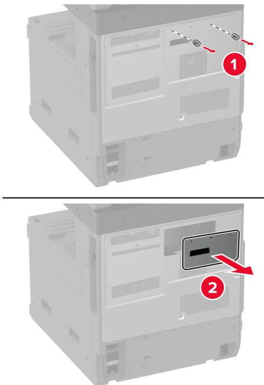
**5** Remove the controller board shield.
