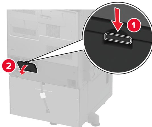
**10** Connect the tray connector to the printer, and then attach the cover.
