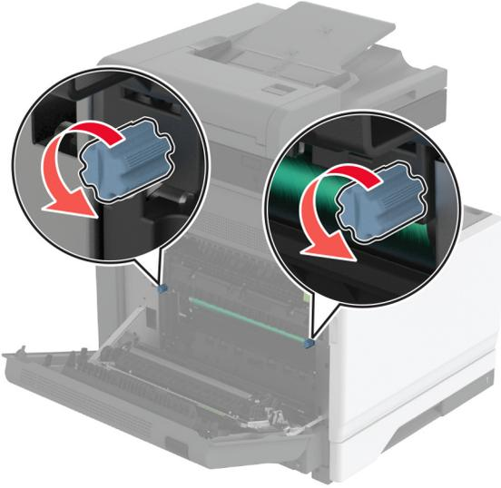
**4** Remove the used fuser.
