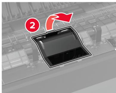
4 Remove the separator roller.
