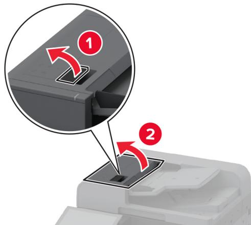
**3** Remove the separator roller cover.
