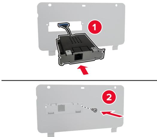
**8** Insert the fax connector cable to the controller board compartment.
