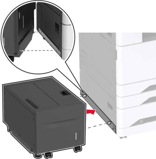
**7** Connect the tray connector to the printer.
