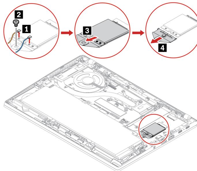
**Note:** During installation, ensure that you connect the cables with different colors to the corresponding connectors on the card according to the illustrations above: the orange cable to the connector labeled ORANGE, the blue cable to the connector labeled BLUE, the white and grey cable to the connector labeled WHITE GREY, and the black and grey cable to the connector labeled BLACK GREY.
