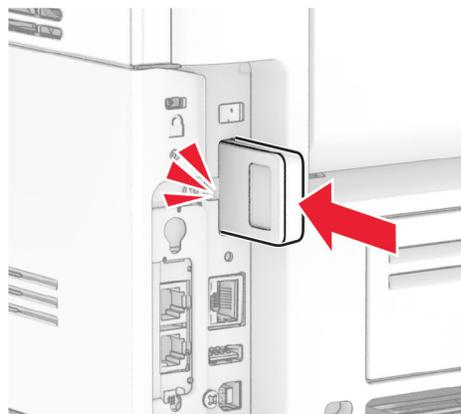
**9** Insert the fax card, and then install the screws.
