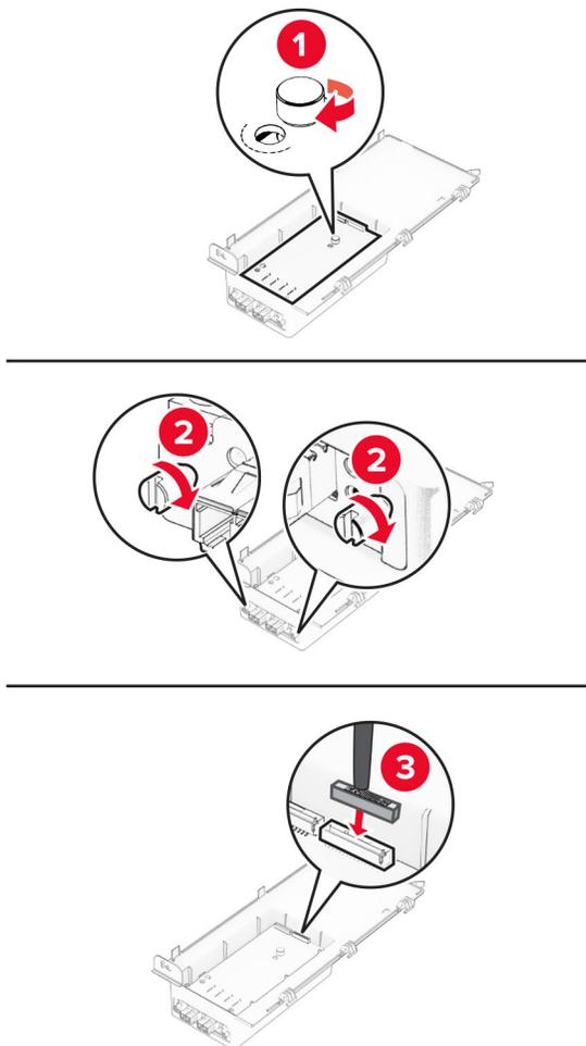
**7** Using a flat-head screwdriver, remove the controller board access cover.
