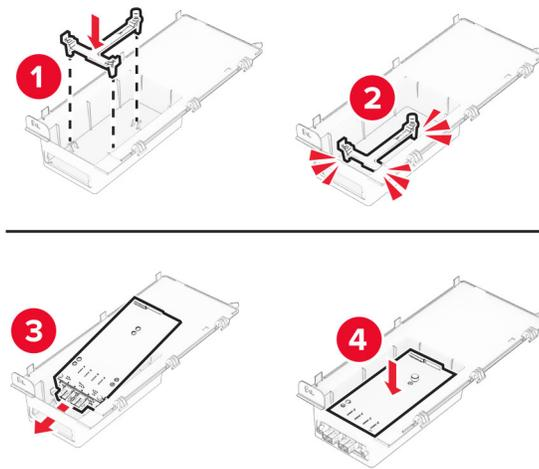
**6** Secure the ISP in place, and then attach the ISP extended cable.
