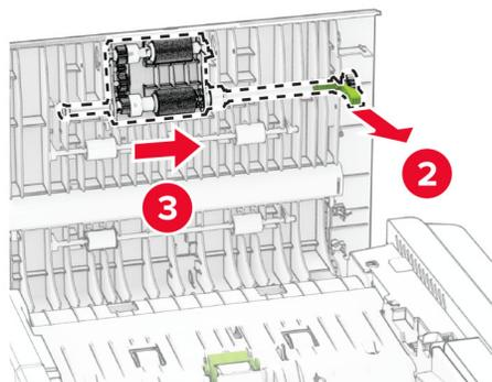
**3** Remove the used ADF separator roller.
