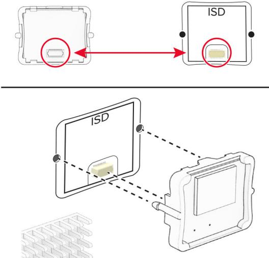
**8** Install the fax card, and then install the screws.
