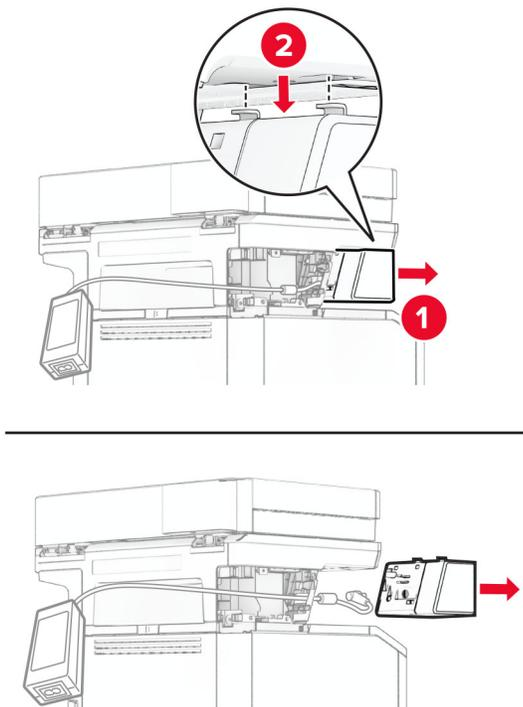
**6** Remove the used power supply.
