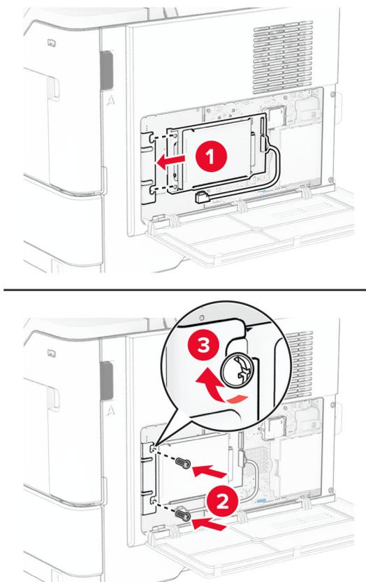
**6** Attach the hard disk interface cable to the controller board.
