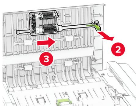
**3** Remove the ADF separator roller.
