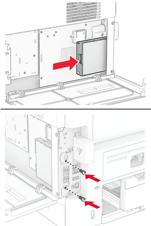
**10** Attach the wireless print server cover, and then install the screw.
