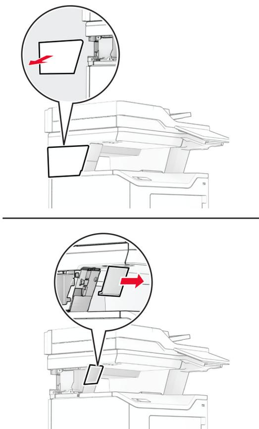
**5** Insert the power supply through the printer, and then connect it to the convenience stapler.
