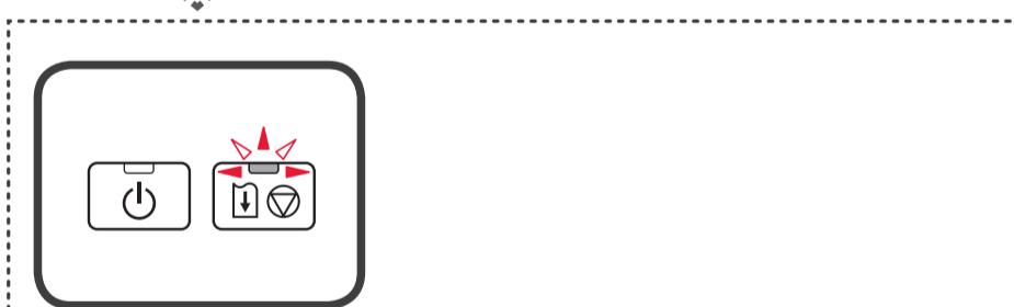
If the **Alarm** lamp flashes, check that the Print Head and ink tanks are installed correctly.
