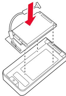
**6** Attach the hard disk to the controller board shield.
