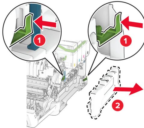
**Note:** To avoid spilling the toner, place the bottle in an upright position.
