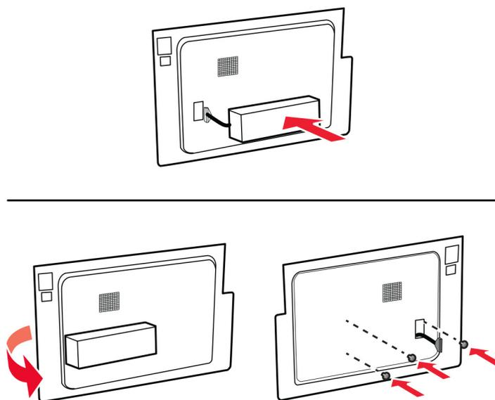
**7** Connect the hard disk interface cable to the controller board.
