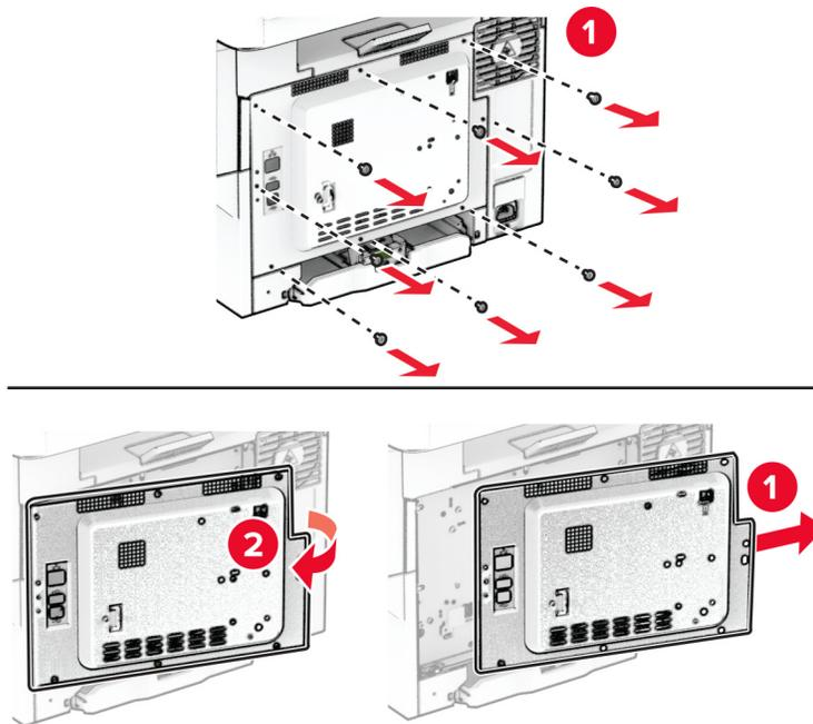
**4** Remove the hard disk port cover from the controller board shield.
