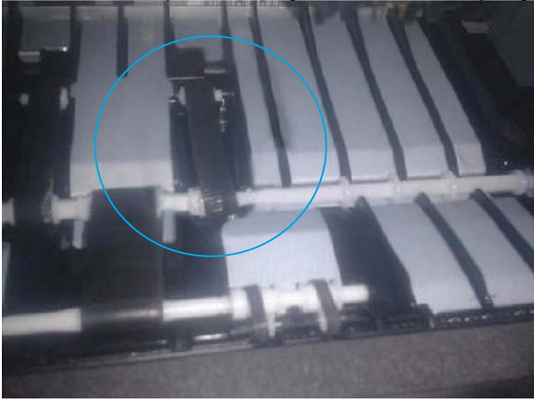
8. If belt is extremely loose and will not stay centered when printing, replacing the Paper Feed Assembly.
