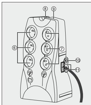
shut down the **UPS** (button (8) OFF), remove the power cord (2) and proceed as indicated below.
