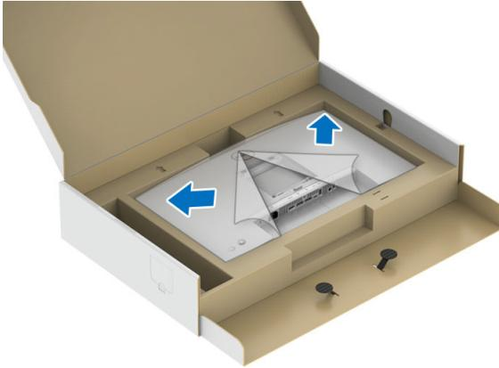
6. Attach the stand assembly to the monitor.
