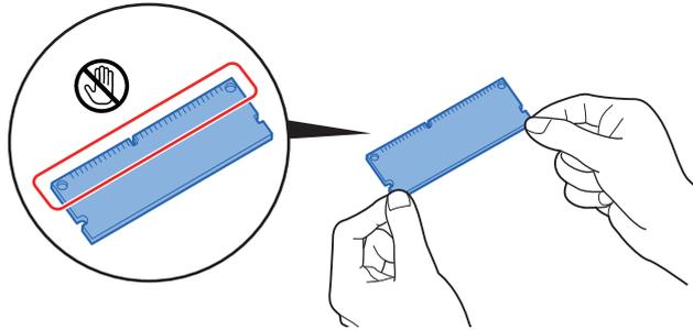
To protect electronic parts, discharge static electricity from your body by wearing an antistatic wrist strap, if possible, when you install the memory modules. If you do not have a wristband, touch a metal object to discharge static electricity before inserting the memory.
