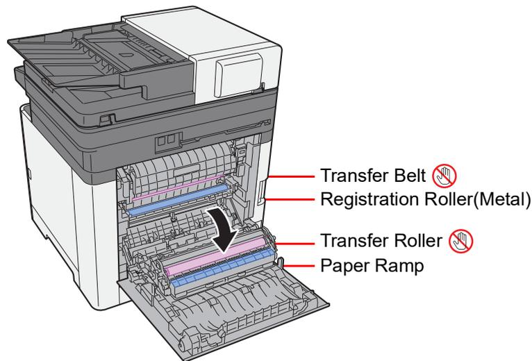
Wipe away the paper dust on the registration roller and the paper ramp using the cloth.
