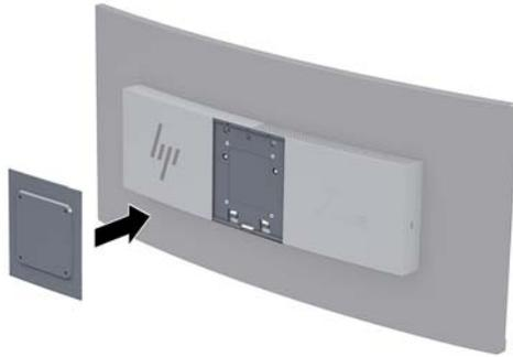
4. To attach the monitor to a swing arm or other mounting device, insert four mounting screws through the holes on the mounting device and into the screw holes on the VESA bracket.
