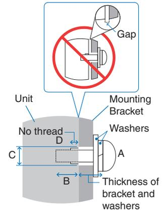
**NOTE:** When used in a video wall configuration for a long time, slight expansion of the monitors may happen due to temperature changes. It is recommended that a gap of over one millimeter is kept between adjacent monitor edges.
