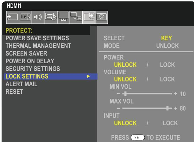
1. Using the remote control, navigate to [PROTECT] then to [LOCK SETTINGS].
