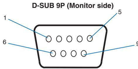
This monitor uses RXD, TXD and GND lines for RS-232C control.
