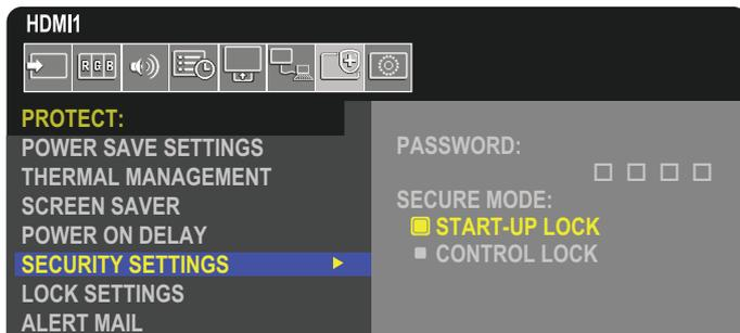
1. Using the remote control, navigate to [PROTECT] then to [SECURITY SETTINGS].
