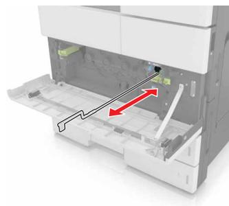
5 Remove the printhead wiper.
