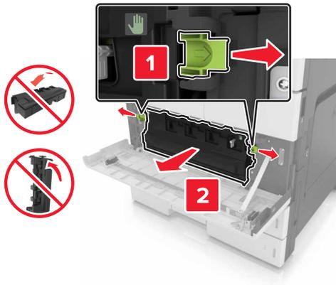
3 Unlock the photoconductor unit.
