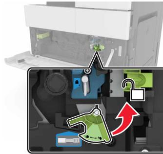
4 Remove the photoconductor unit.
