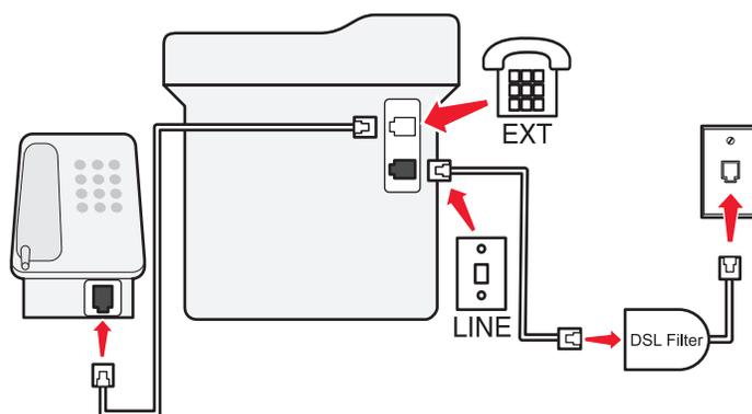
A Digital Subscriber Line splits your regular telephone line into two channels: voice and Internet. Telephone and fax signals travel through the voice channel, and Internet signals pass through the other channel. This way, you can use the same line for analog voice calls (including faxes) and digital Internet access.
